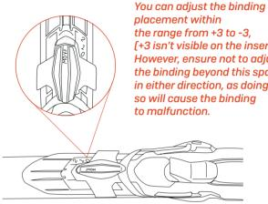
With Rottefella MOVE Tune, you can move your binding easily and quickly, and fine-tune your bindings based on snow conditions, the terrain and your technique.
