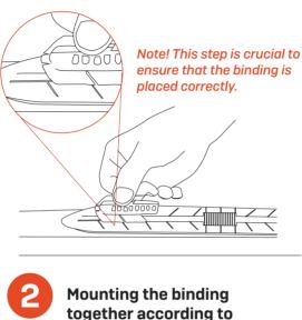
Turn the binding housing and heel plate with the underside facing up. Insert the heel plate into the binding housing at an angle as shown in step 1 below. When the forks on the heel plate is beneath the tabs on both sides of the binding housing, rotate the heel in place (step 2). Press down until you hear a click.
