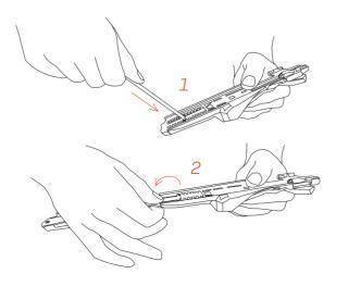
Mounting the SkateX binding onto the mounting plate
