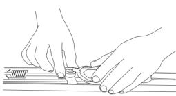
Push the binding forward until it stops. Turn the handle counter clockwise as shown in the illustration below, as you continue pushing the binding forward.
